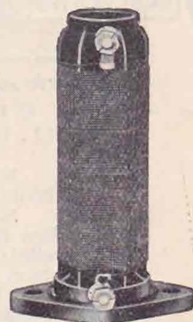
No. 923—Short-wave H.F. Choke. Space wound. 9-100 metres to carry 40 m. amps.
